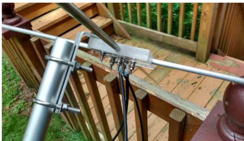
Figure 4 — The turnstile is attached to the mast with two U bolts and a 90-degree aluminum L bracket.
