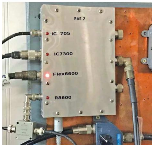
Figure 2 — The RAS2 switch box.
