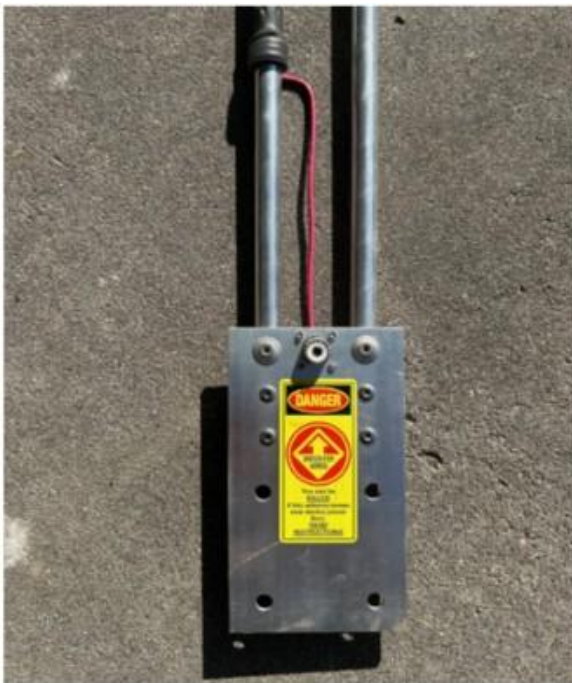
Figure 2 — The tubing mounts to the plate with pop rivets. An SO-239/UHF connector mounts on the same plate and feeds the longer element through the matching wire.
