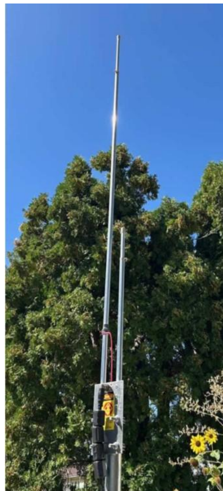
The deployed Adjust-a-J antenna.
