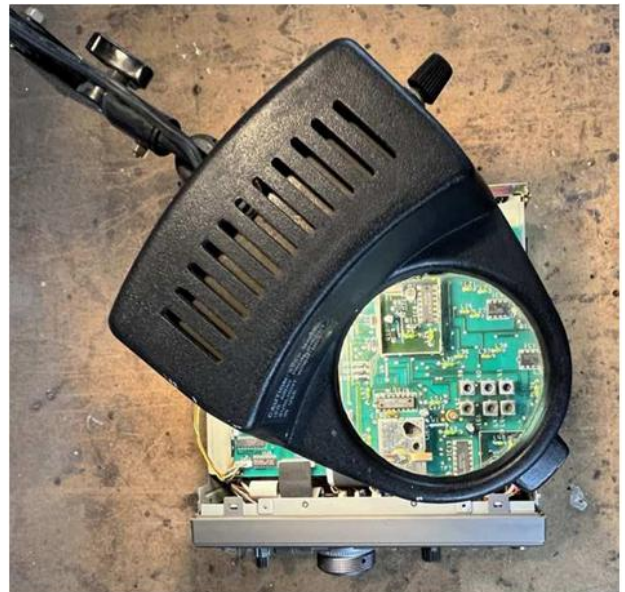
Figure 2 — An illuminated magnifier helps improve visual inspections.
