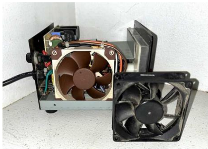
Figure 1 — Sumner Weisman, W1VIV, replaced the cooling fan in his MFJ switching power supply.
