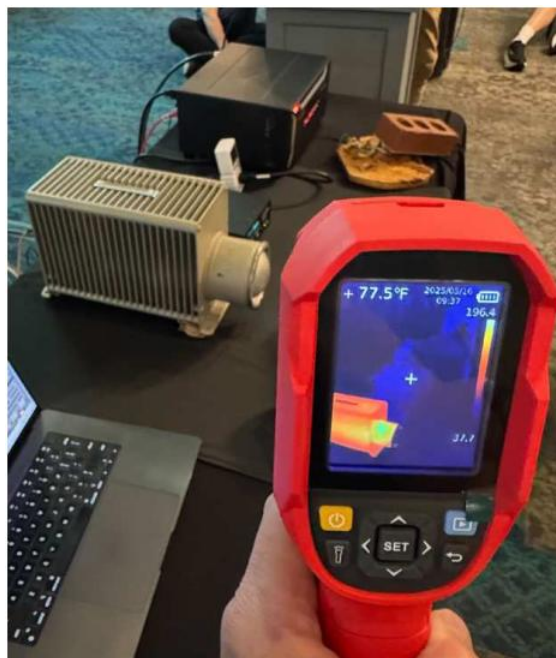
A demonstration of polar modulation’s heat efficiency. A brick placed on the CW key in the background had been causing it to transmit for more than 48 hours, and the transmitter’s temperature never reached high levels. [Michael Walker, VA3MW. photo]
