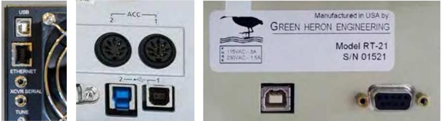
Figure 2 — The back of an Elecraft KPA1500, an Icom IC-7610, and a Green Heron RT-21 showing the USB-B port.
