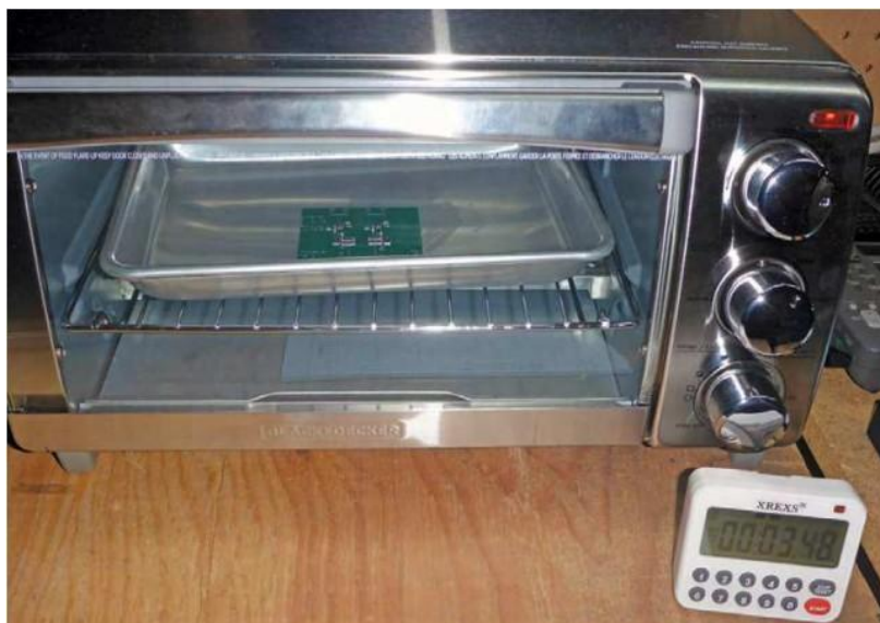
Figure 5 — The toaster oven soldering station.
